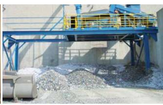
Since glass is highly abrasive on conveyor belts and equipment, it is removed first and stored outside until it is shipped.
