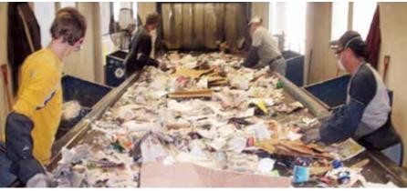
**PRE-SORT LINE:** The sorters remove items that may harm or interfere with equipment such as plastic bags, large metal items and trash.
